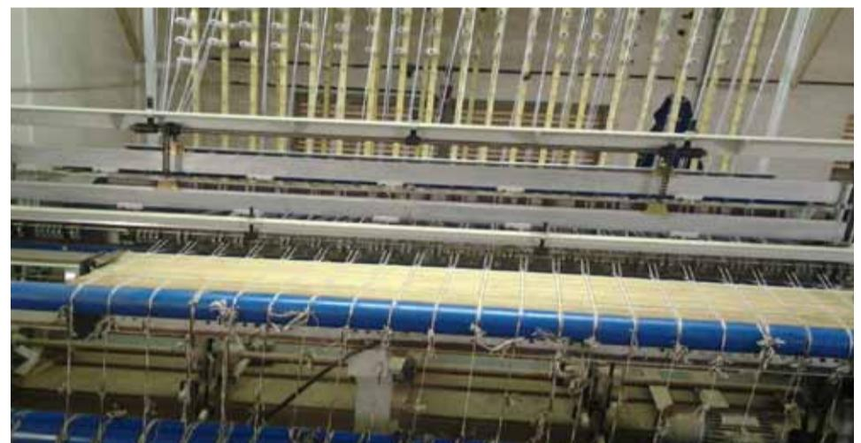
Electronic weaving machine used to make bamboo wall curtains illustrated in KEFRI Karura
